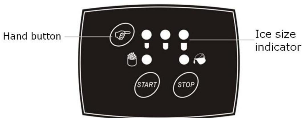
1. Select the size of the ice by pressing the "HAND" button. If the room temperature is lower than 60°F, it is best to select the small or medium ice size, otherwise the ice might stick together.
